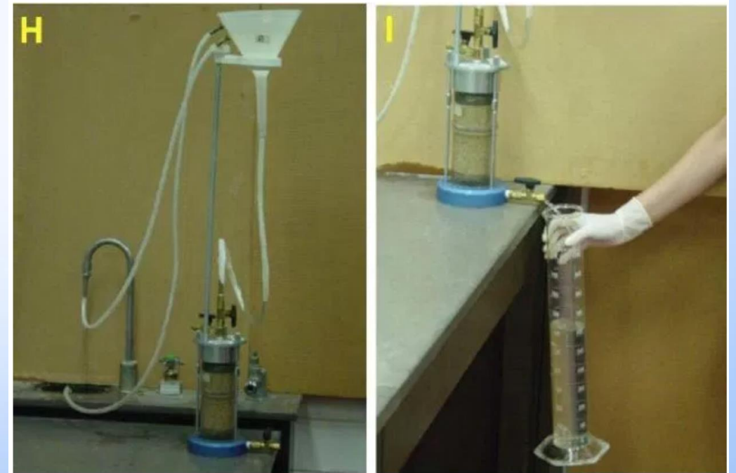
Figure 3. Hydraulic Conductivity Test [2]
