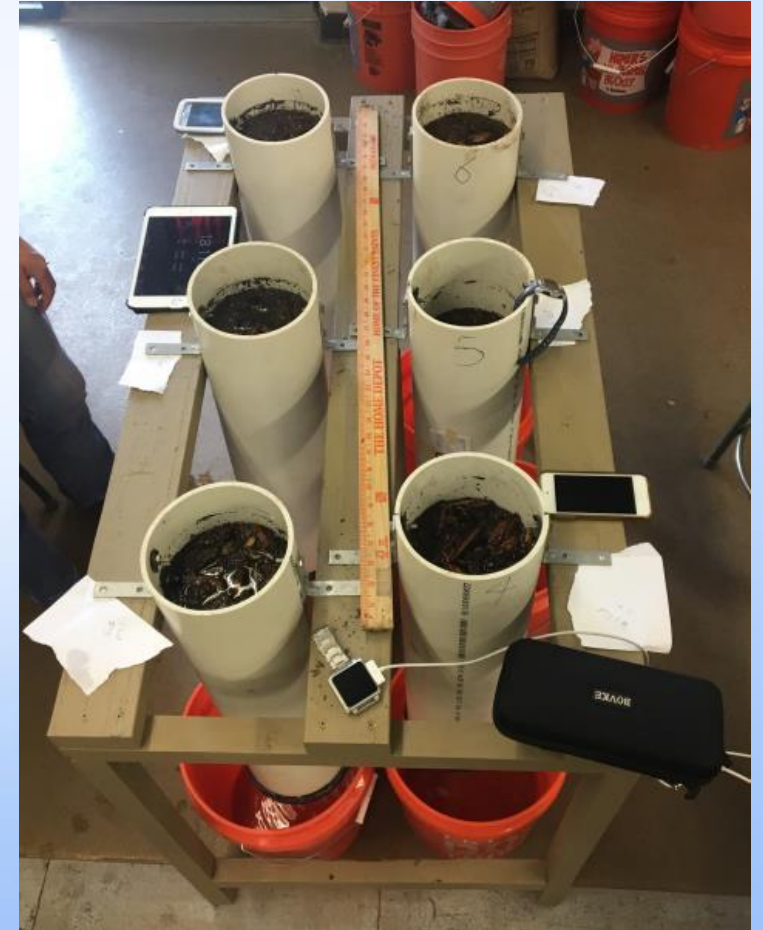
Figure 4. Soil Matrix Infiltration Testing Method [3]
